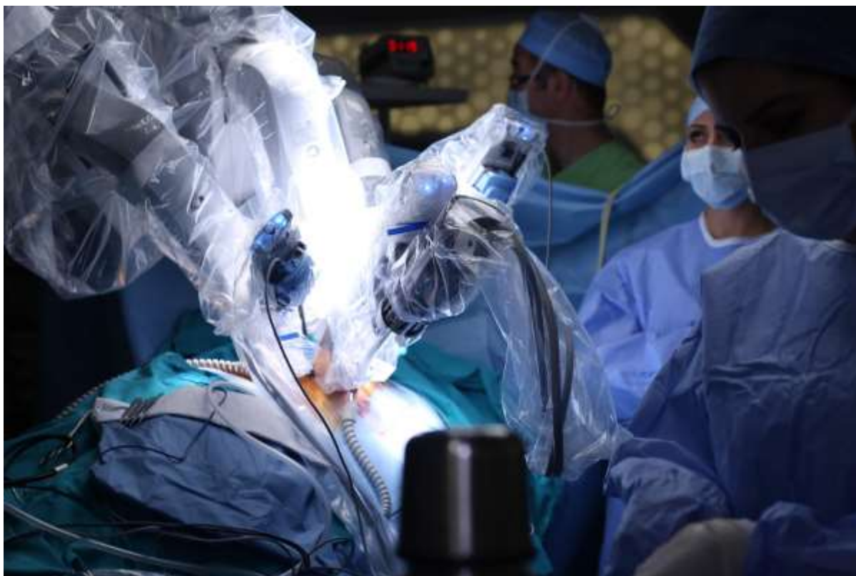
Figure 3: During robotic surgery, the camera and other surgical instruments are operated by the robot, which the surgeon controls from a console [51].
