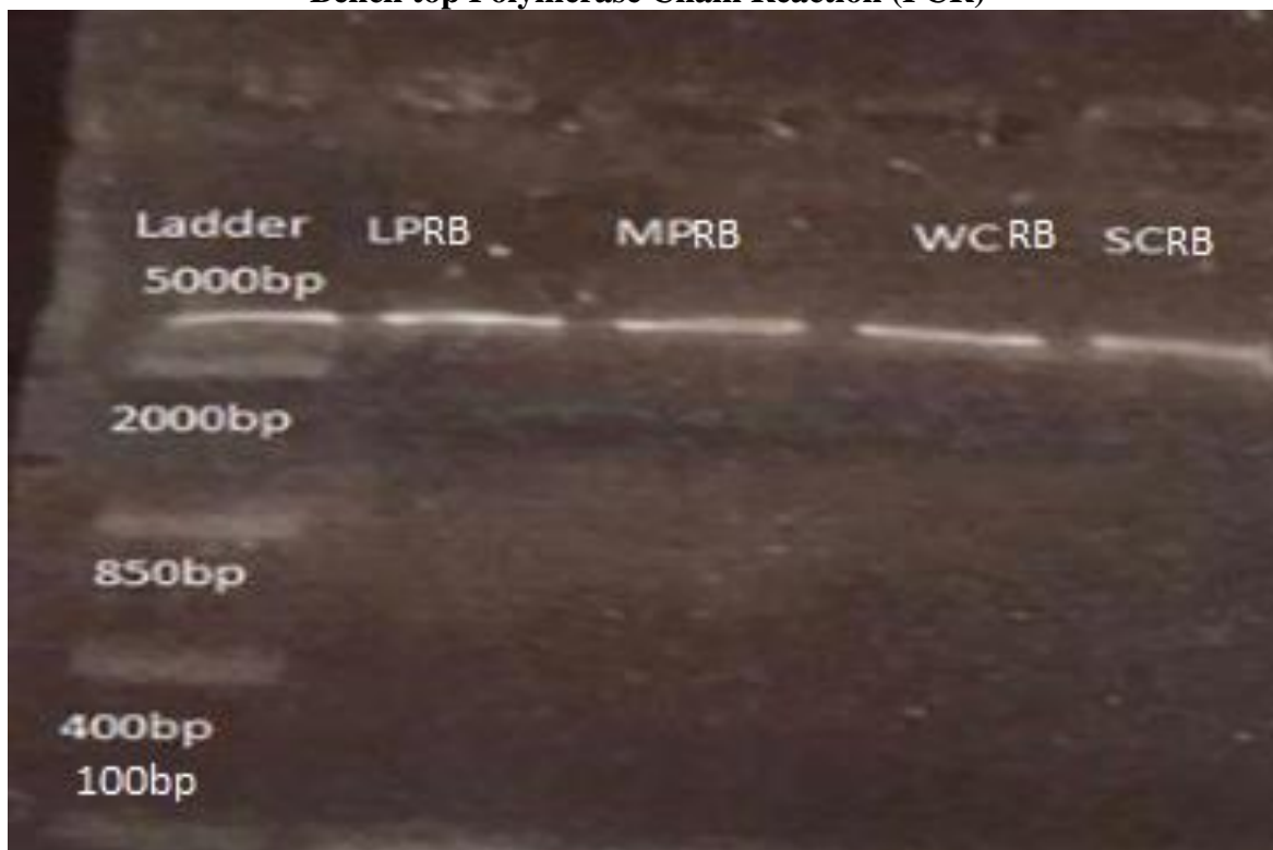
Figure 4: Gel electrophoresis results of four isolates of yeast from rose Bengal agar (yeast extracted genomic DNA). In each row, bands in accordance with 5000bp ladder, shows that the genomic DNA of the yeast was successfully extracted from the yeast cells.
