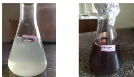
Fig-1 Colour transformation of the 1mM AgNO 3 solution with the addition of P. fruticosa leaf saponin extract
