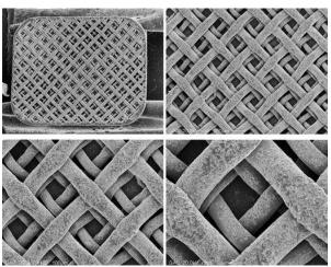
SEM photographs at different magnifications (from  $\times 20$  to  $\times 200$ ) for the Ovation double-mesh bracket bases, in the "as received" condition
