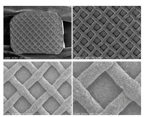
SEM photographs at different magnifications (from  $\times 20$  to  $\times 200$ ) for the Victory single-mesh bracket bases, in the "as received" condition
