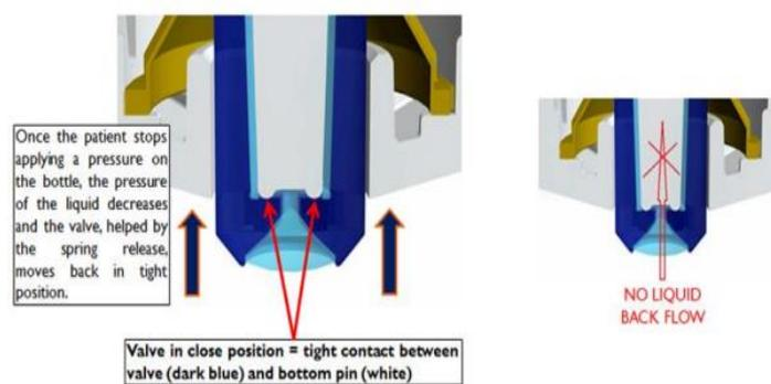
The action of closing the one-way valve breaks the liquid column between the nozzle and the bulk.
