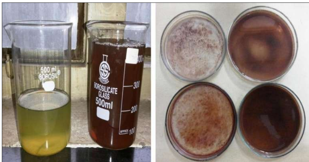
Fig. 2 Synthesis of Spirulina platensis mediated silver nanoparticles: A) Spirulina extract and its nanoparticle solution B) Dried nano powder
