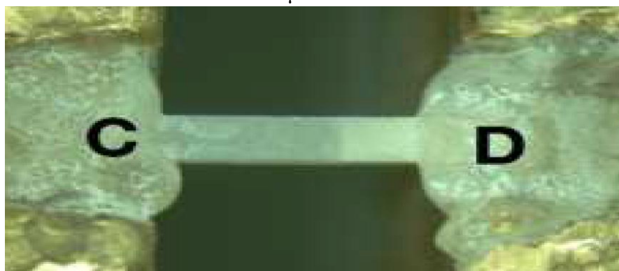
Figure (2): A photograph showing a rod sample was connected to a Geraldelli jig and tensioned from each sample Microtensile tester (C representing composite direction and D representing denting direction).
